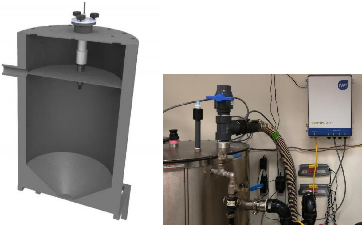
FIGURE 2 THE LEFT IMAGE IS A 3D DRAWING OF THE CUSTOM MOUNT AND BES SENSOR. THE RIGHT IMAGE IS A PICTURE TAKEN OF THE INSTALLED CONTROL PANEL
